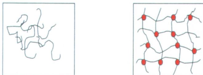
Figure 15.1. Crosslinked vs. non-crosslinked films
